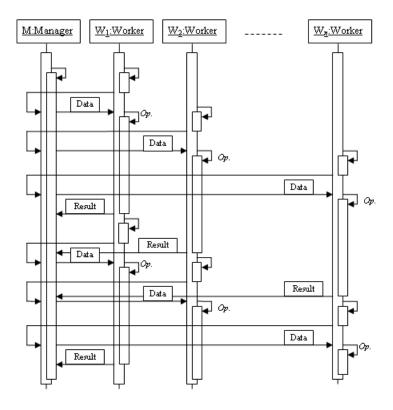
Fig. 2. Interaction Diagram of the Manager-Workers pattern.
